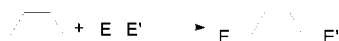
Figure 1. 1,4-Addition of an interelement compound to a 1,3-diene. E,E' = Si, Ge, B or Sn.
